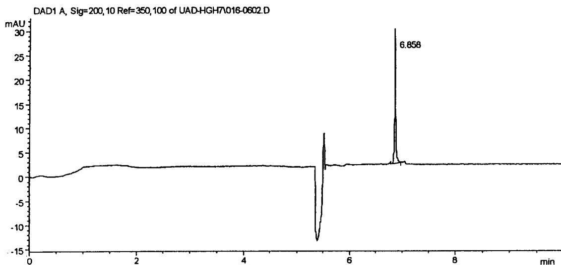
Fig. 13. r-hGH electropherogram. Technical conditions: buffer, \text{NaH}_2\text{PO}_4 - \text{Na}_2\text{HPO}_4 100 mM (pH 8.0); capillary, 560 mm/645 \mu\text{m} , I.D. 50 \mu\text{m} ; voltage and pressure, 25 kV, 23°C, 5 \times 10^{-2} MPa·s (11.8 nl); sample, r-hGH in water (440 \mu\text{g}/\text{ml} ); instrument, Hewlett-Packard 3D CE.
